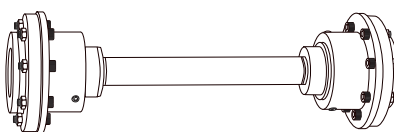
Type T50 Floating Shaft
